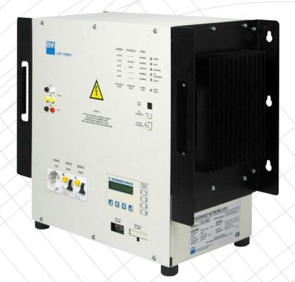
EKA's Broadband Network UPS model FR-1000 replaces outside plant standby power supplies in CATV networks, providing true UPS performance in a high efficiency package. The power module will retrofit most standby enclosures enabling any system to upgrade easily. The FR-1000 architecture incorporates an inherent "soft start" feature eliminating any need for high-inrush circuit breakers and nuisance breaker tripping.
